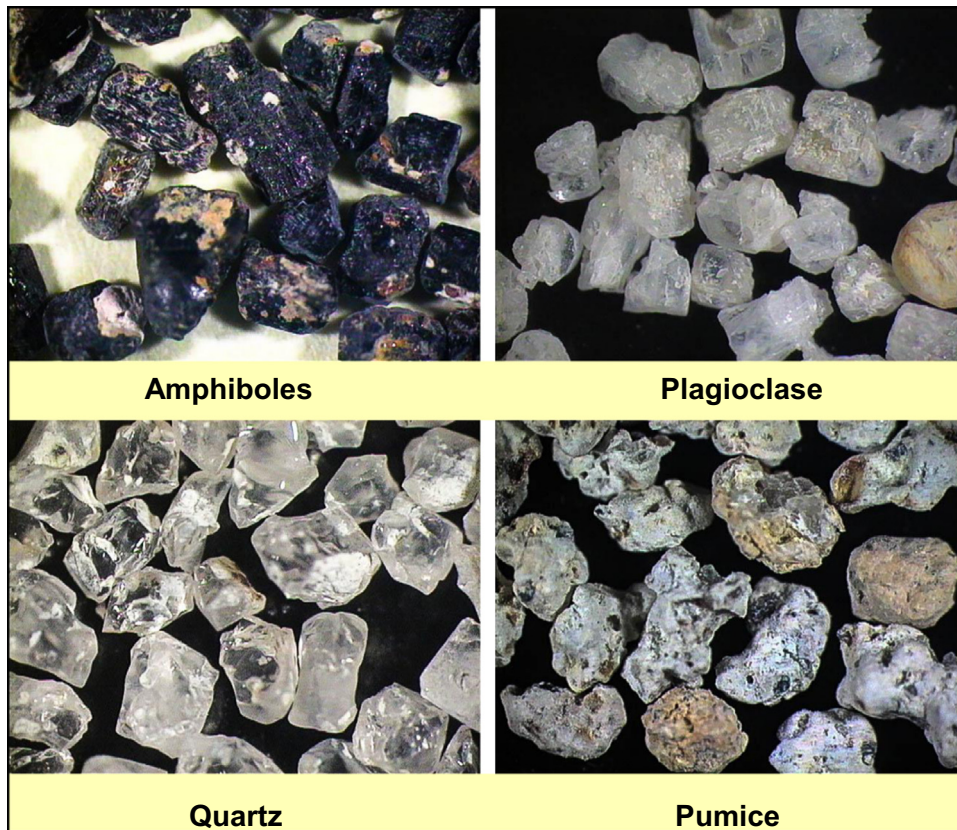
Fig. 4. Four types of minerals identified in volcanic soil samples. (For interpretation of the references to color in this figure, the reader is referred to the web version of this article.)
