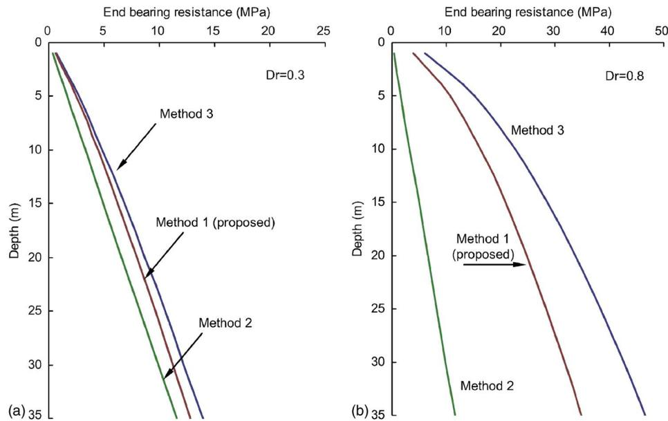
Fig. 6. Predicted end bearing resistance of piles in (a) loose sand and (b) dense sand
