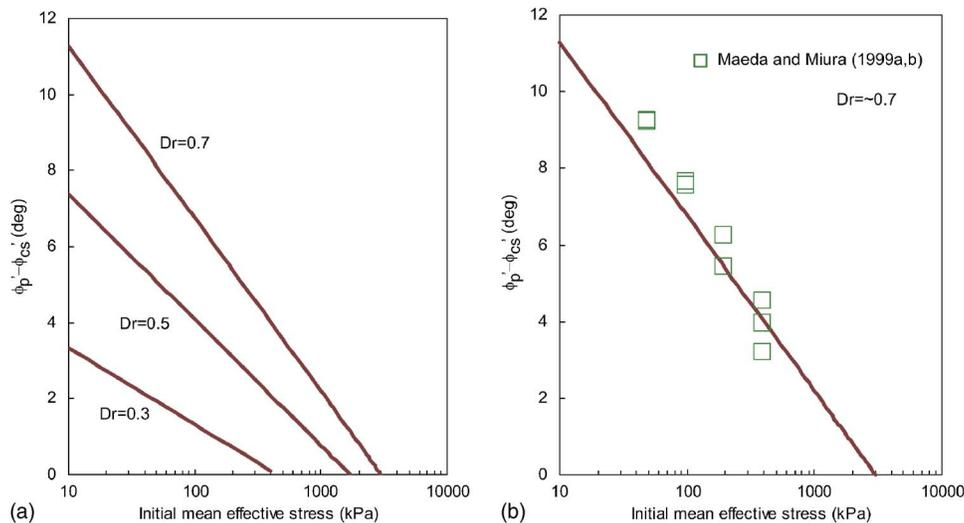
**Fig. 2.** State-dependent effective friction angle: (a) prediction; (b) prediction versus experimental data
