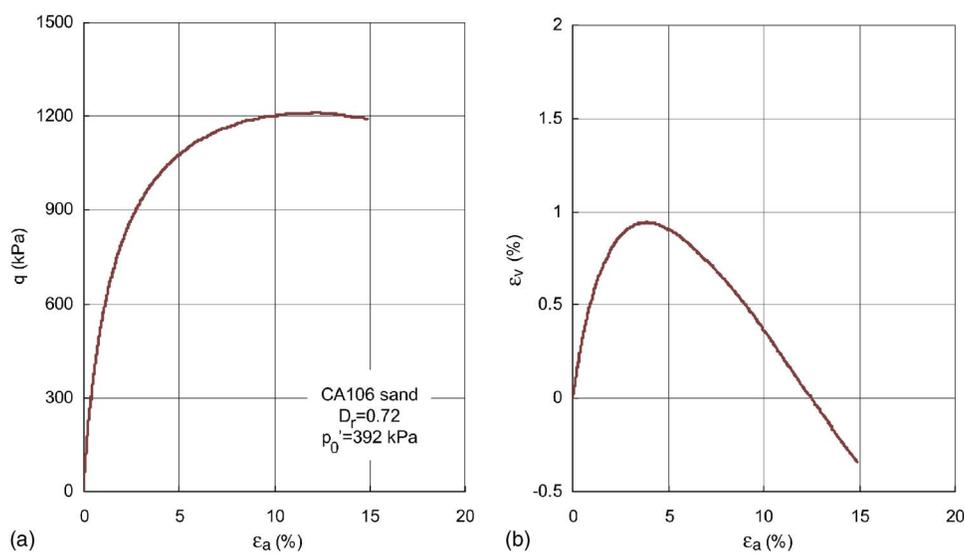
**Fig. 4.** Response of a medium dilatant sand in triaxial compression (data courtesy of K. Maeda): (a) stress–strain behavior; (b) volumetric behavior
