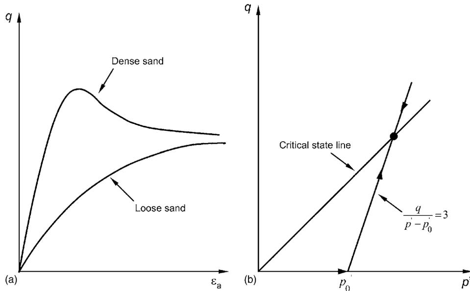
**Fig. 1.** Typical response of sand in triaxial compression tests: (a) stress–strain behavior; (b) stress path
