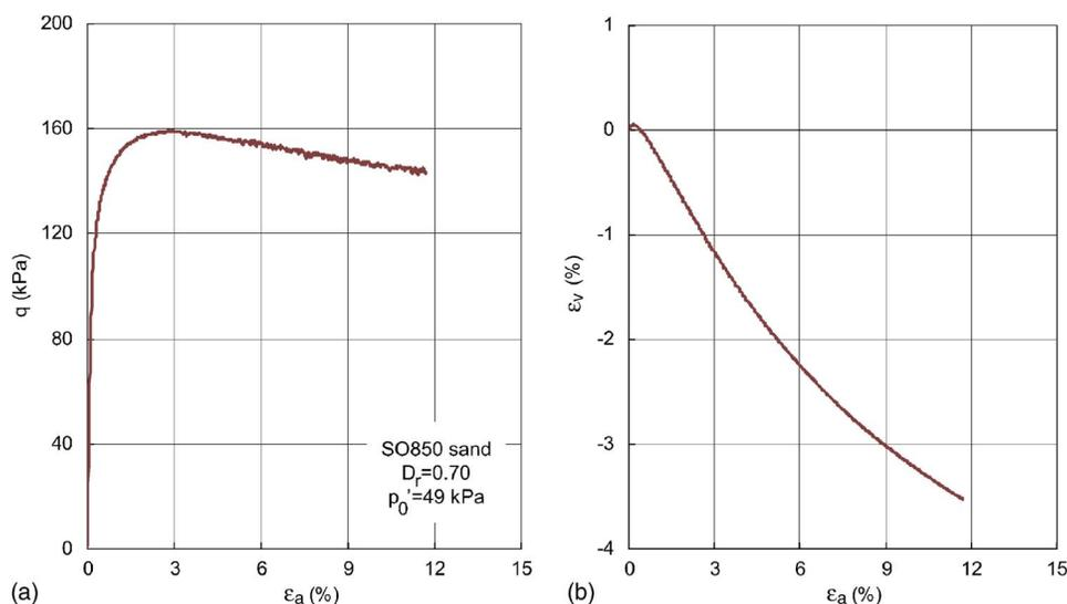
**Fig. 3.** Response of strong dilatant sand in triaxial compression (data courtesy of K. Maeda): (a) stress–strain behavior; (b) volumetric behavior
