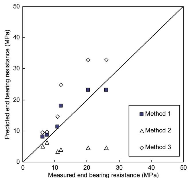
**Fig. 5.** Predicted and measured end bearing resistance of test piles
