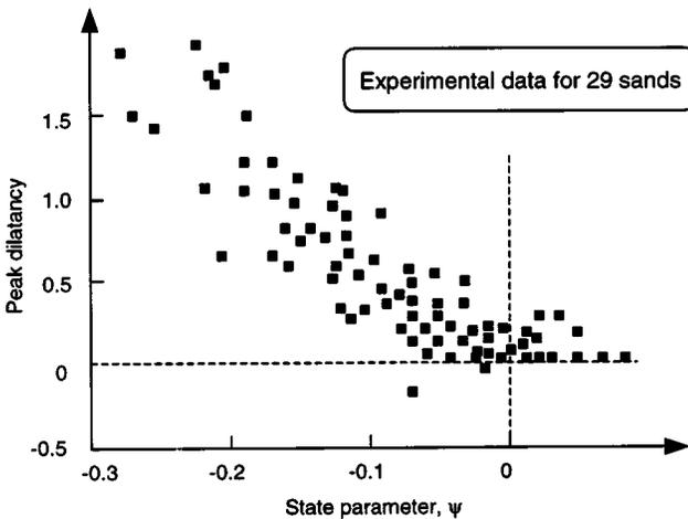
**Fig. 17.** Experimental data of relations among peak friction angle, maximum dilation, and state parameter (after Been and Jefferies 1986 and Been et al. 1992)
