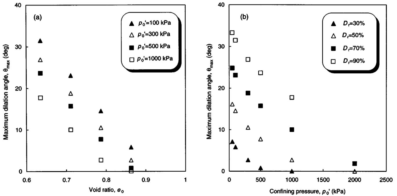
Fig. 15. Influence of density and stress level on maximum dilation angle
