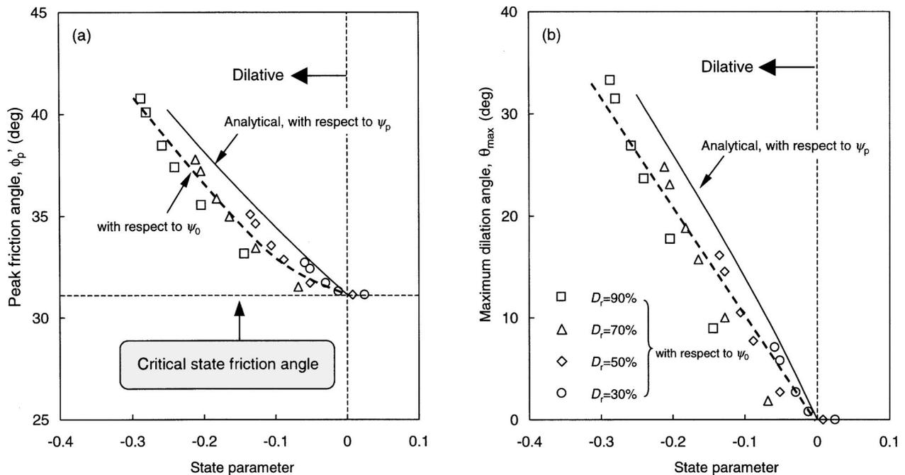
Fig. 16. Peak friction angle and maximum dilation angle as function of state parameter
