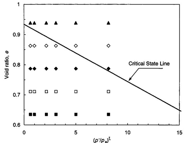
Fig. 4. Initial states of Toyoura sand covered in analyses
