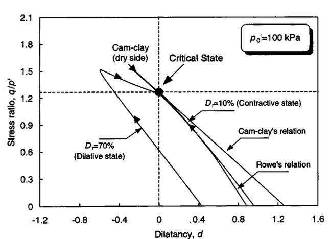
**Fig. 10.** Development of stress ratio with dilatancy for sand with different confining pressures and densities
