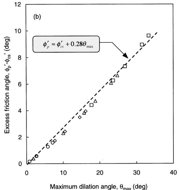
**Fig. 18.** Relationship between peak friction angle and maximum dilation angle
