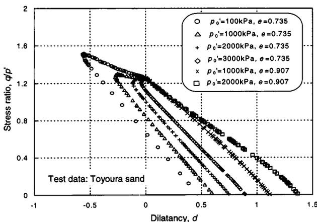
**Fig. 11.** Experimental data of stress-dilatancy relation (data from Verdugo and Ishihara 1996)
