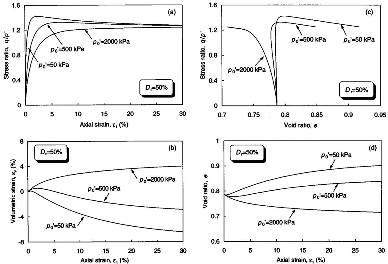
Fig. 6. Typical stress–strain response and volume change characteristics of sand with different confining pressures
