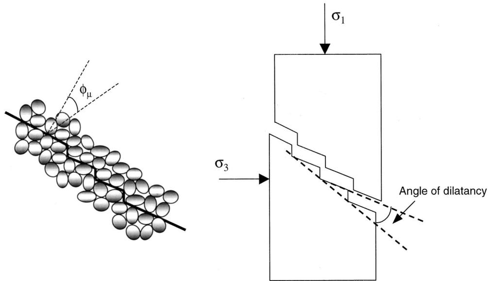
Fig. 2. Sliding mechanism assumed for Rowe's stress-dilatancy theory
