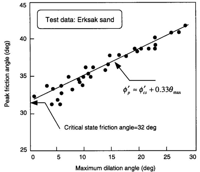
**Fig. 19.** Test data of relationship between peak friction angle and maximum dilation angle (after Vaid and Sasitharan 1992)
