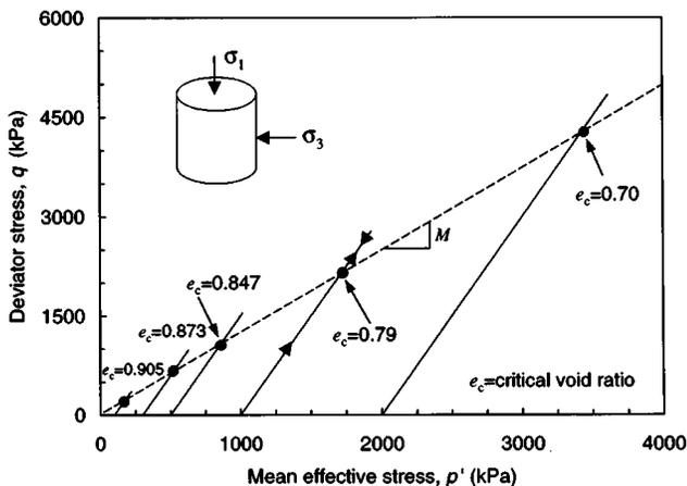
Fig. 5. Typical stress paths involved in analyses
