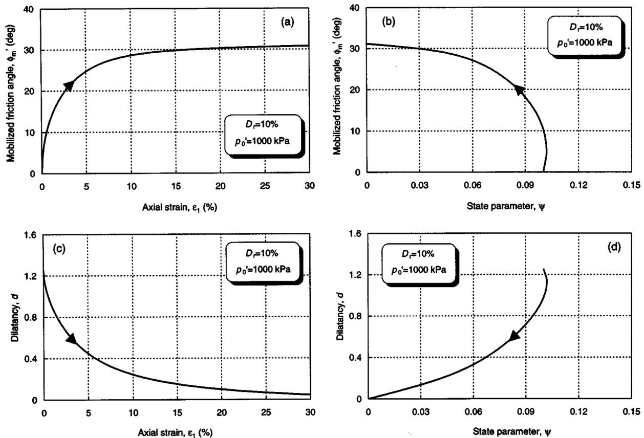
Fig. 9. Evolution of mobilized friction angle and dilatancy for loose state
