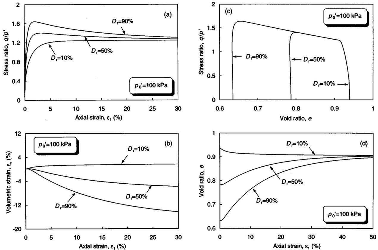
Fig. 7. Typical stress–strain response and volume change characteristics of sand with different initial densities
