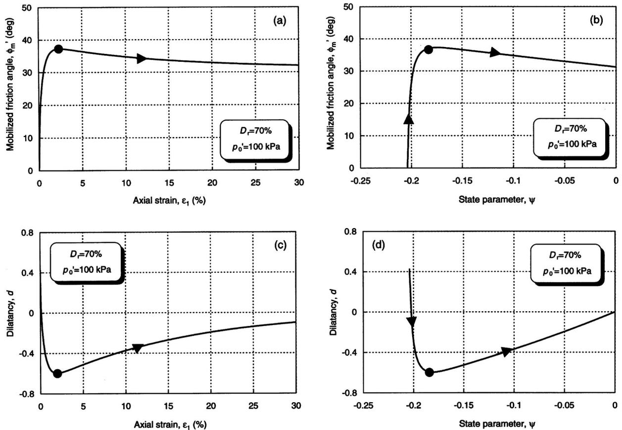
Fig. 8. Evolution of mobilized friction angle and dilatancy for dense state
