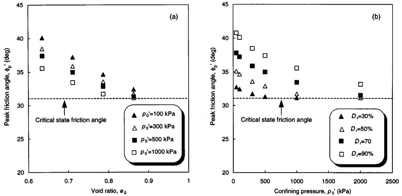
Fig. 13. Influence of density and stress level on peak friction angle
