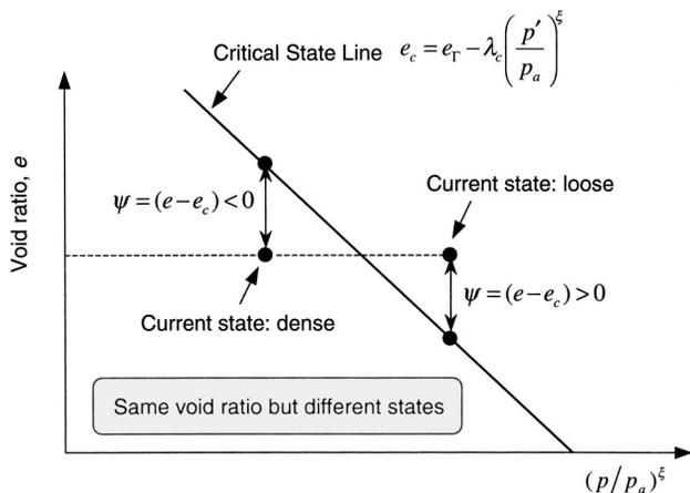
Fig. 3. State parameter and critical state line
