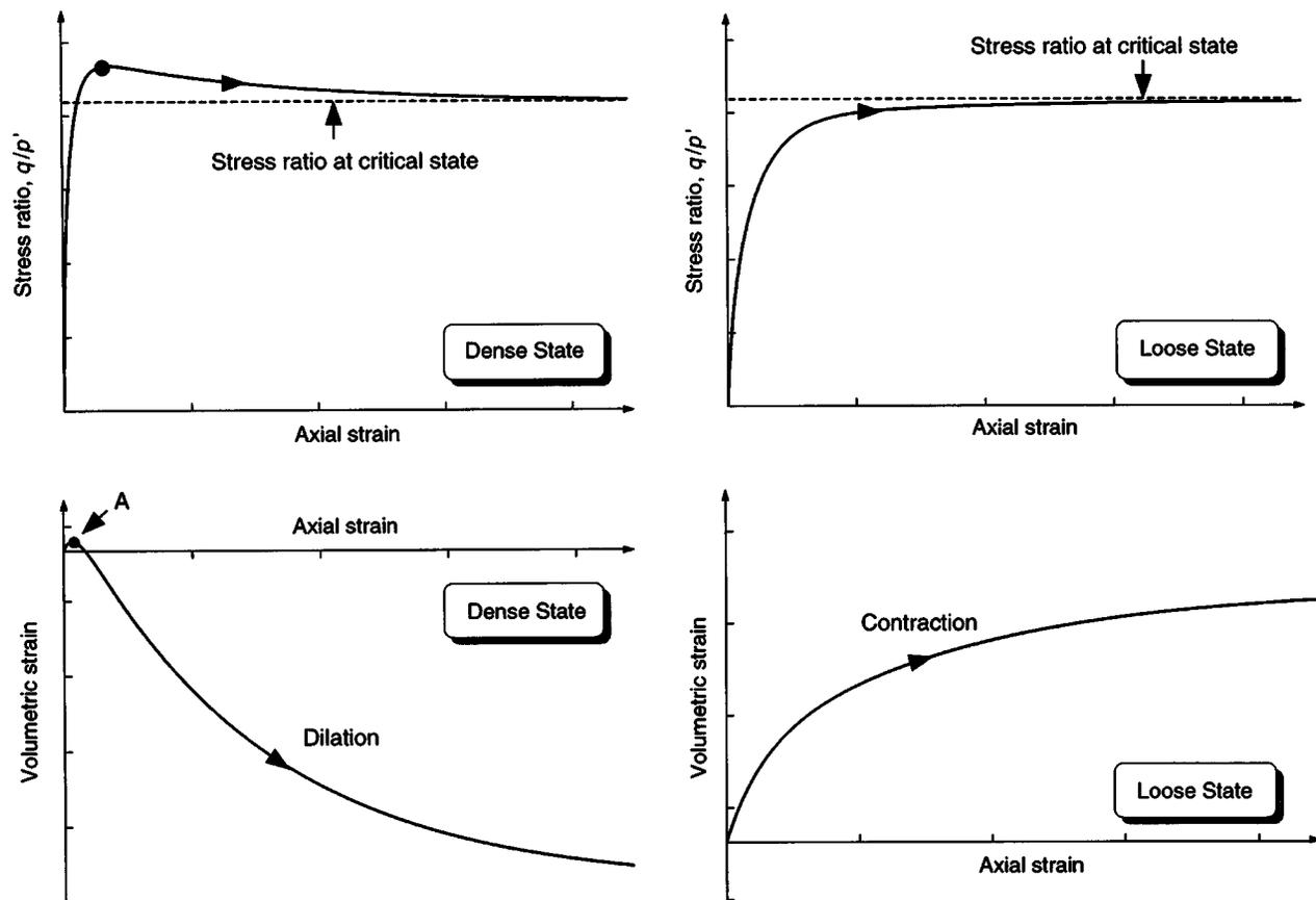
Fig. 1. Typical response of sand in loose and dense states in triaxial compression
