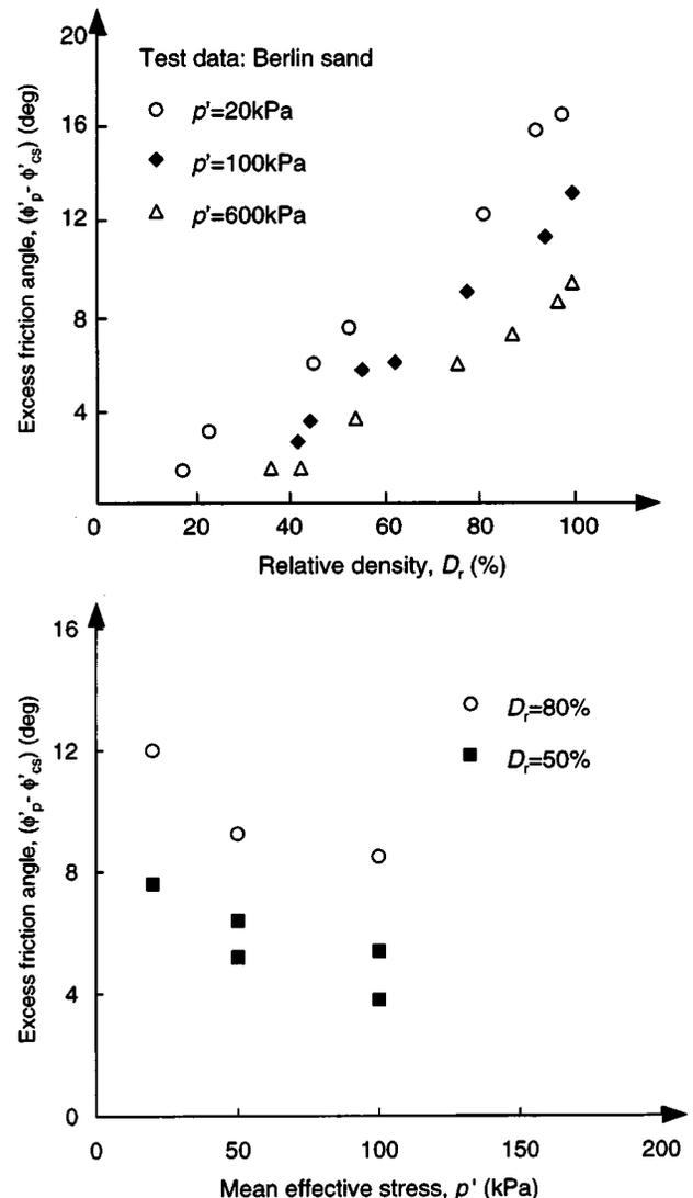
Fig. 14. Test data for density and pressure dependent friction angle (data from De Beer 1965)
