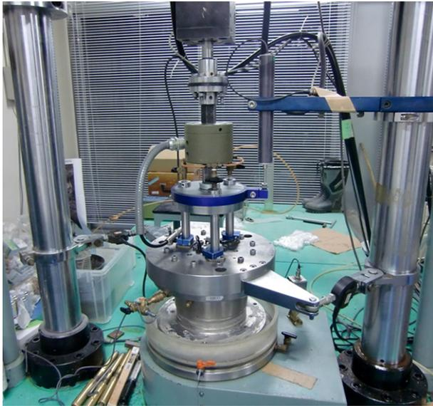
Fig. 2. An overall view of the ring-shear apparatus DPRI-Ver.5.
