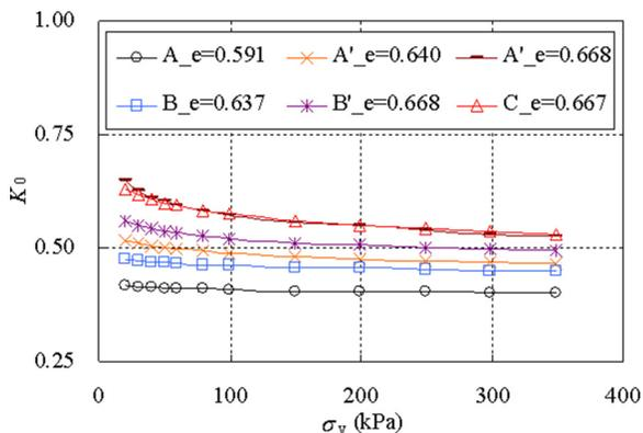
Fig. 3. Effects of confining pressure and void ratio on the  $K_0$
