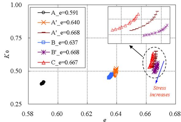
Fig. 4. Relationship between the  $K_0$  and void ratio
