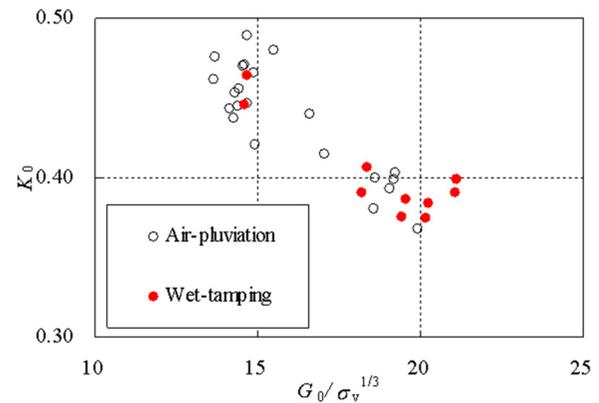
**Fig. 8.** Relationship between the  $K_0$  and normalized small strain shear modulus for Toyoura sand in the laboratory ( $G_0$  in megapascals and  $\sigma_v$  in kilopascals)
