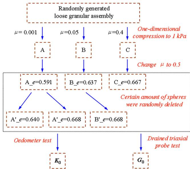
Fig. 2. Schematic diagram of the DEM simulation
