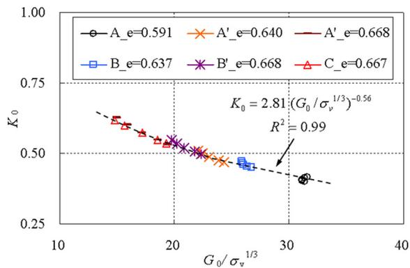
**Fig. 7.** Relationship between  $K_0$  and normalized small strain shear modulus in the DEM ( $G_0$  in megapascals and  $\sigma_v$  in kilopascals)
