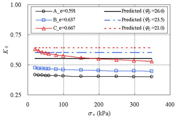
**Fig. 6.** Comparison of  $K_0$  obtained by DEM simulation and predicted by Jaky's equation
