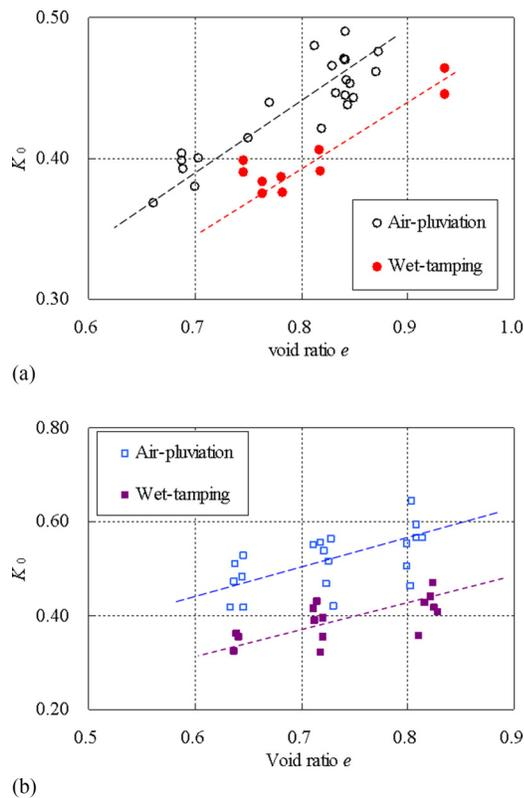
**Fig. 1.** Effect of void ratio and sample preparation method on the  $K_0$  [(a) data from Okochi and Tatsuoka 1984; (b) data from Northcutt and Wijewickreme 2013]
