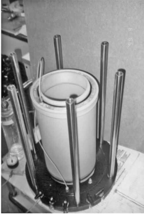
Fig. 2. Set-up of a hollow cylindrical sample
